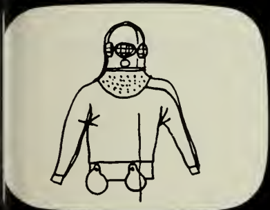
AUGUSTUS SIEBE'S 1819 "open dress" was successful forerunner of modern gear. Pumped air escaped at waist.
